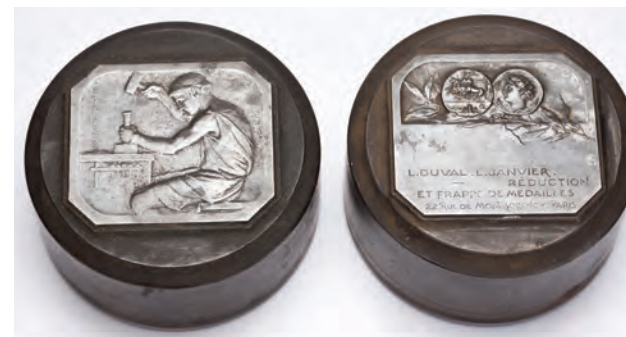
Fig. 8: France. Pair of Hubs made for L. Duval & L. Janvier. Iron. (ANS 2013.43.1–2, gift of David Gladfelter) 90 x 40 mm (images reduced).
