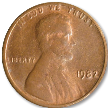
This 1982 Lincoln cent shows a case of peripheral die expansion and erosion. Peripheral letters are truncated where they meet the design rim.
