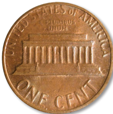
This 1982 Lincoln cent shows a case of peripheral die expansion and erosion. Peripheral letters are truncated where they meet the design rim.
