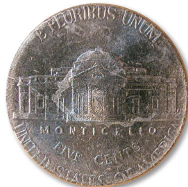
The reverse face of this 2014-P 5-cent coin shows a case of design creep. The reverse (hammer) die face expanded radially, beyond the working face of the collar.
